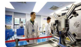
Barcode DOF Testing System
